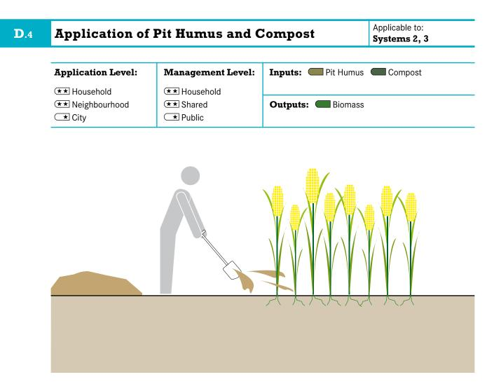
Compost is the soil-like substance resulting from the controlled aerobic degradation of organics. Pit humus is the term used to describe the material removed from a double pit technology (S.4, S.5 or S.6) because it is produced passively underground and has a slightly different composition than compost. Both products can be used as soil conditioners.
